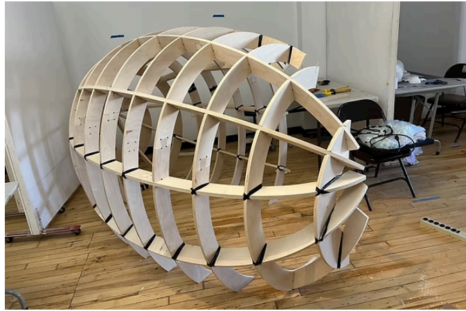
Fig. 14: The cocoon's shell by CNC (2022), material is birch plywood.
